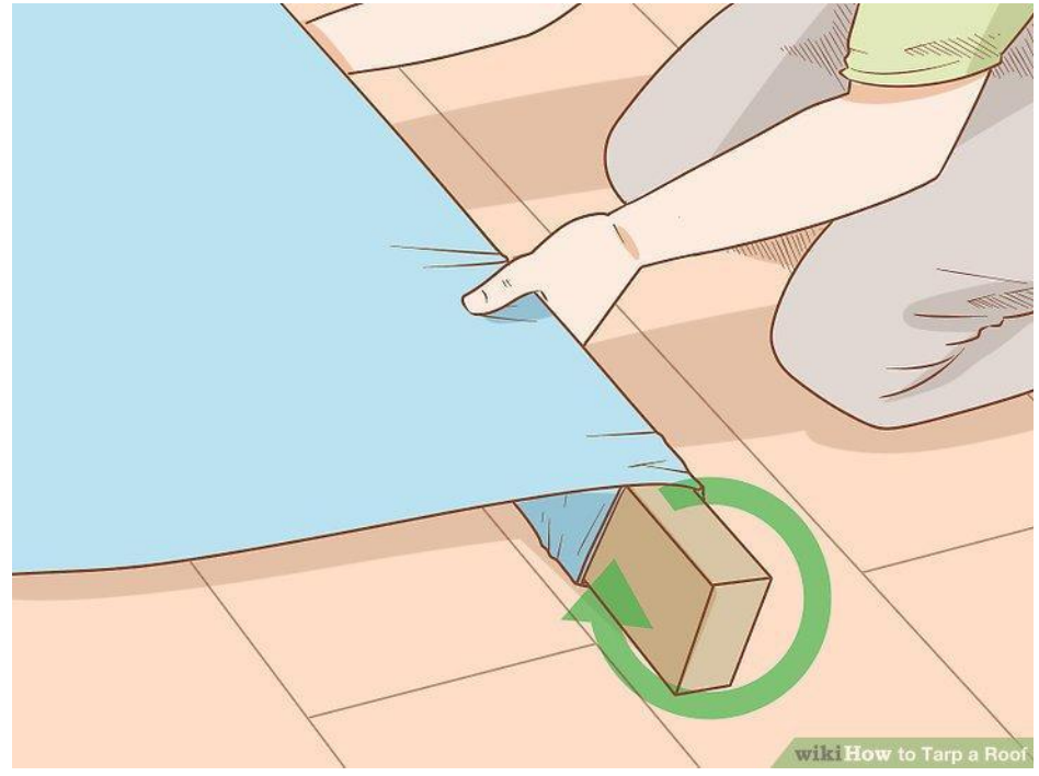
Roll the 2x4 as shown to strengthen the connection to avoid tarp tearing
